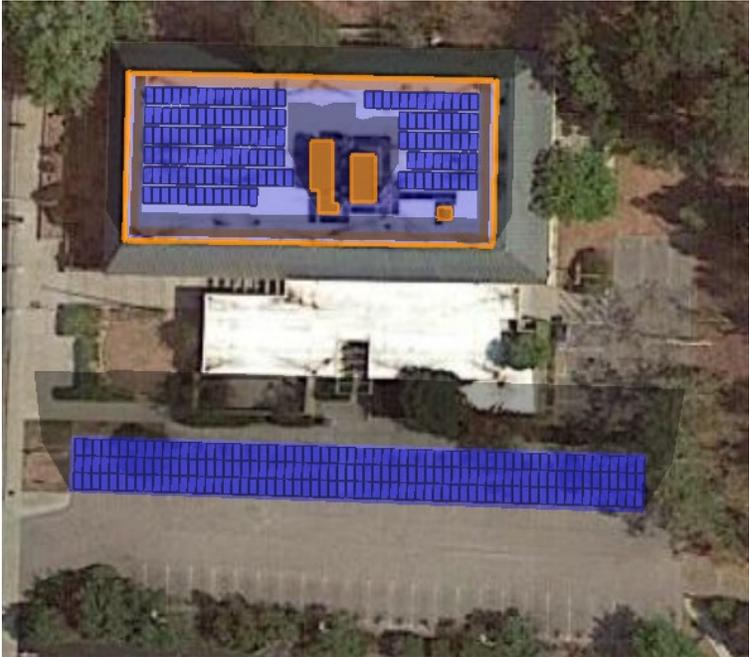
The layout above can accommodate approximately 50 kW on rooftops and 68 kW of solar carports in parking lots, for a total of 118 kW. The energy yield for proposed solar arrays is 1619 kWh/kW per year.
