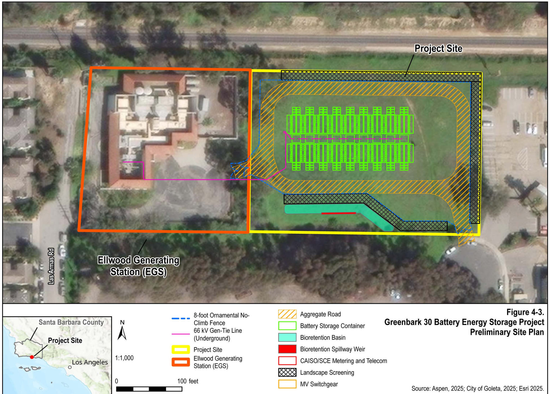
Figure 4-3. Greenbark 30 Battery Energy Storage Project Site Plan
